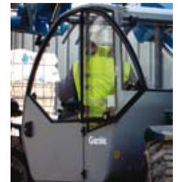
DOOR WITH 2 SECTIONS: STEEL ON BOTTOM, GLASS ON TOP. BOTH SECTIONS OPEN SEPARATELY.
