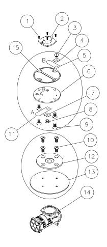
*CAUTION:* Depending on the product, the vacuum system may require the valve plate (6) to be rotated to an orientation different from the one shown. When removing the valve plate, always take note of its orientation in the pump head (2), and install the valve plate the same way during reassembly. In all cases, the valve plate must be oriented so that its intake hole is matched with the head port that connects to the check valve.
